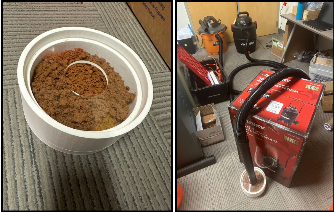
Figure 3: Muck cavity filled with soil (left), Full V0 muck removal test setup (right)
